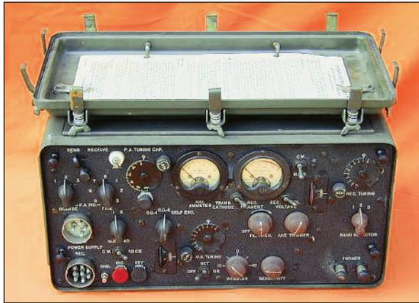
This is the transmitter/receiver part of the TBX-6 radio used by the Code Talkers. The transmitter portion is on the left and the receiver portion on the right. [Antonio Fucci, I8000PU SWL, [www.radiomilitari.com](http://www.radiomilitari.com), photo]
